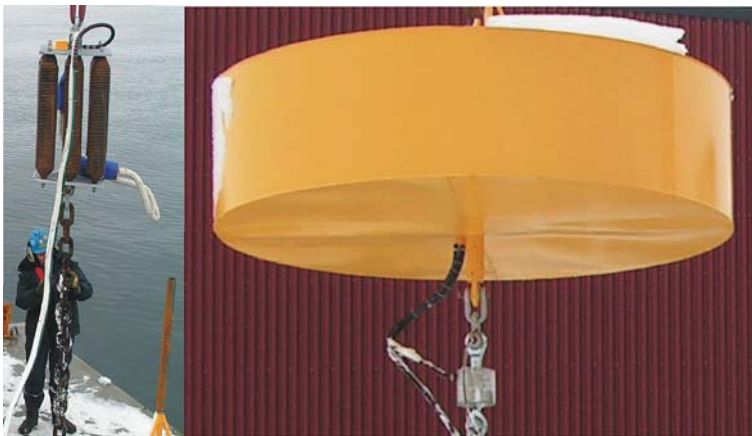
Fig. 3 The packet of springs to the left, the force transducer below the buoy to the right
